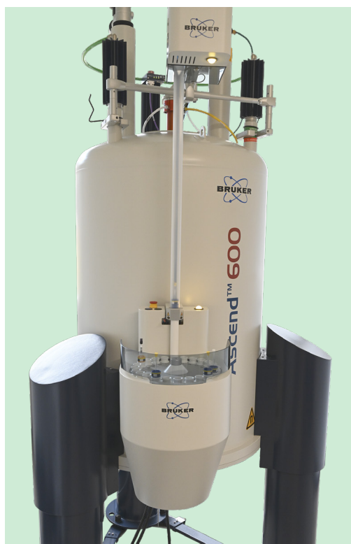
Bruker ASCEND 600 MHz NMR magnet system.
